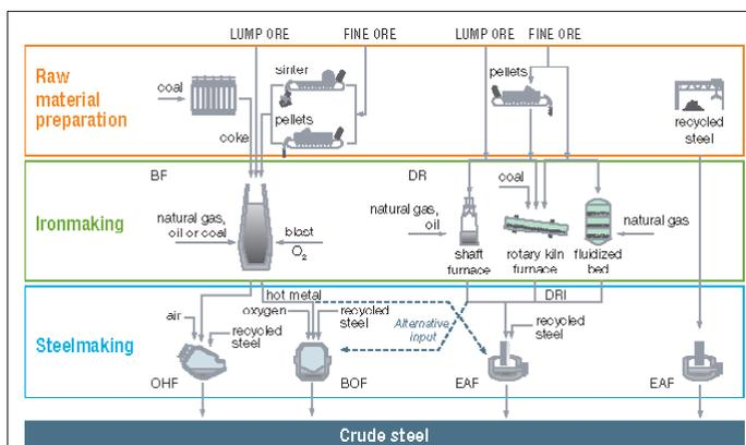
Figure 1: Steelmaking routes
