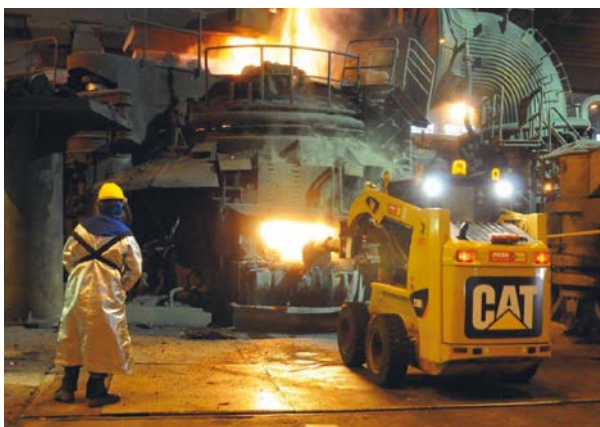
Breast cleanliness: removal of the operator from the risk area. Gerdau Steel Mill – Charqueadas, Rio Grande do Sul, Brazil
